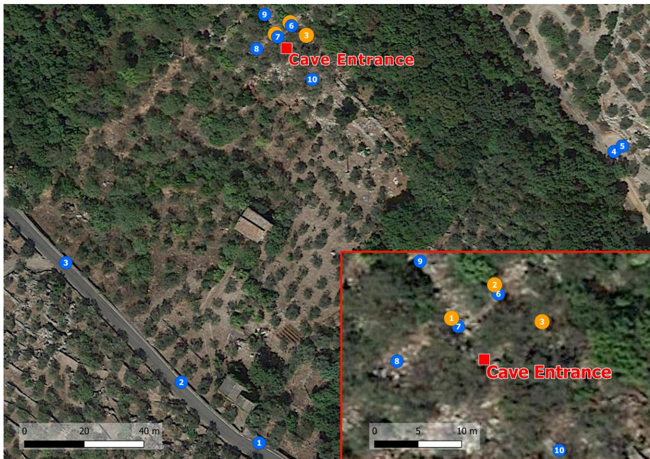
Figure 1 – The GCP acquired for the internal (orange) and outside (blue) survey
