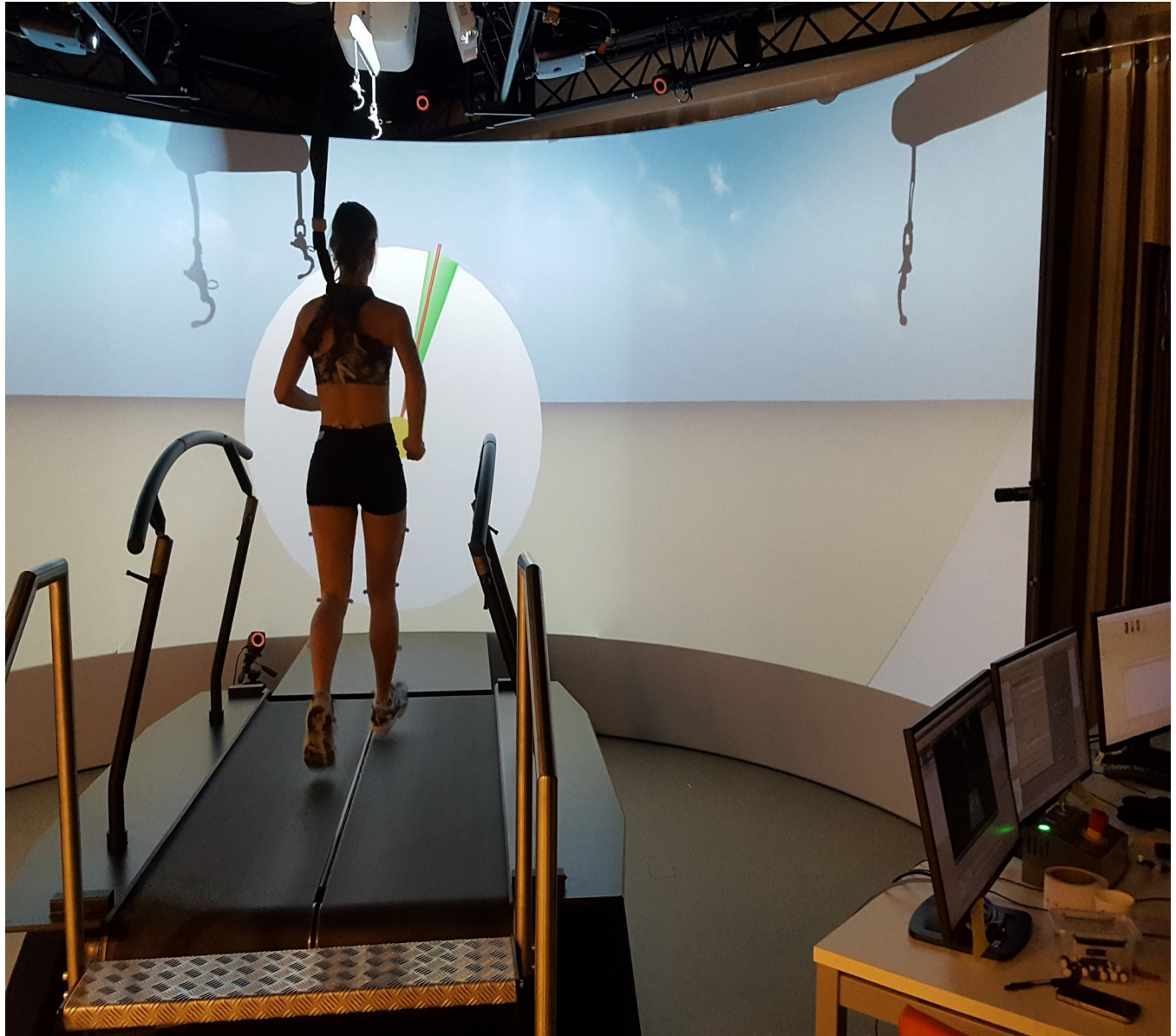
Fig 2. Picture representing real-time visual feedback for changing FPA. The training process: Real-time visual feedback is provided to the subject via the big screen. The red pointer represents the FPA of the right foot that is fixed in the midstance (50% stance phase) and updated on each step. The target area is a wedge with a 5^\circ range, with its middle point specifying the subject's normal FPA +5^\circ for toe-out and -5^\circ for toe-in. The aim is to turn the target area green (positive feedback) by keeping the red pointer (FPA) inside the target area. If the red pointer leaves the target area, the target area turns red (negative feedback).
