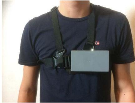
Figure 7.2 | Ambient conditions box with temperature and humidity sensors and data receiver and storage.
