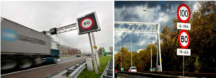
Figure 1.1. Left, a single dynamic road sign which can display e.g. both a speed limit of 80km/h or 100 km/h, dependent on relevance for each specific moment in time. Right, the multitude of fixed road signs that is needed to convey the same message. Both are examples from the Netherlands.
