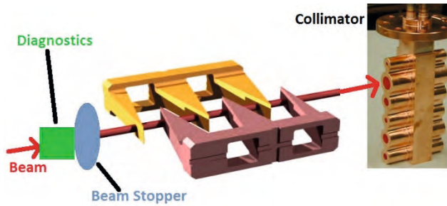
Figure 1.3: The carbon-wedge degrader unit consisting of its diagnostics, a beam stopper, pair of multi-wedges, and a collimator system [4].
