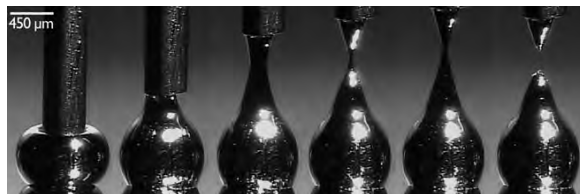
Figure 1.9 | A series of photographs of the formation of a conical tip of EGaIn. From left to right: a micromanipulator i) brings a drop of EGaIn suspended from the needle of a syringe into contact with the bare, reflective surface of a Ag film, and ii) raises the syringe until the EGaIn separates into a conical tip (which remains attached to the needle of the syringe) and a drop on the Ag surface. The pictures are sequential and show the formation of a single tip; the time spanned by this sequence is less than 5s. Reprinted with permission from Ref. [153]. Copyright 2008 Wiley-VCH.
