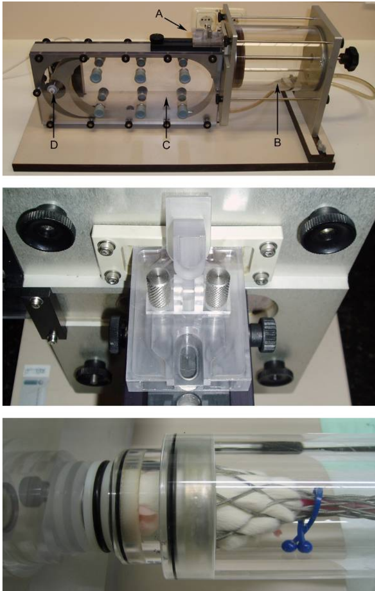
Figure 1. (Top) The aerosol box, a utility for the Twincer ® (A). By pulling the piston in the cylinder (B) an aerosol is created and can be transferred to the exposure chamber (C) to which 12 small laboratory animals can be fitted. A fan (D) creates a laminar airflow in the exposure chamber to minimize sedimentation effects. (Middle) Detail of the Twincer ® attached to the aerosol box. (Bottom) Detail of mouse attached to exposure chamber.
