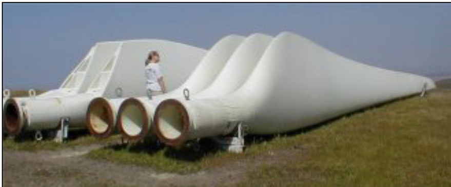
Figure III.3: 15 m blades for Altamont Pass, Ca (photo: Alex Haag)
