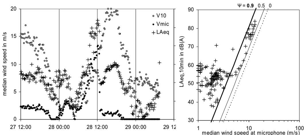
Figure VIII.7: measurements during a storm in front of a big shed; left: 10 minute averages of wind speed at microphone and at 10 m height and sound pressure level  $Leq$ ; right:  $Leq$  as a function of microphone wind speed and predicted sound pressure level ( $G(4.6) = 8.2$  dB)
