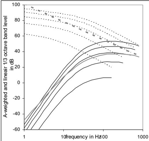
Figure VIII.2: calculated linear (dashed) and A-weighted (solid lines) 1/3-octave pressure levels due to atmospheric turbulence on a screened microphone with  $F(z)+C=42 \text{ dB}$ ,  $D = 0.1 \text{ m}$  and wind speeds 2, 4, 6, 8, 10 m/s (black, bottom to top); bold grey lines: 1/3 octave band levels according to Strasberg for 10 m/s
