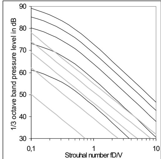
Figure VIII.1: black lines: calculated 1/3 octave band levels  $L_{at,1/3}$  due to atmospheric turbulence at wind velocities of (bottom to top) 2, 4, 6, 8 and 10 m/s;  $F(z) = -18$  dB; gray lines: levels at same wind velocities according to Strasberg
