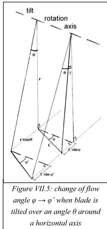
Figure VII.5: change of flow angle  $\varphi \rightarrow \varphi'$  when blade is tilted over an angle  $\theta$  around a horizontal axis
