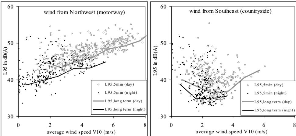
Figure VII.3: 5-minute  $L_{95,5min}$  in day (open, grey diamonds) and night time (solid, black dots) and long-term  $L_{95}$  (lines) as a function of 10-m wind velocity in open terrain for two different wind directions
