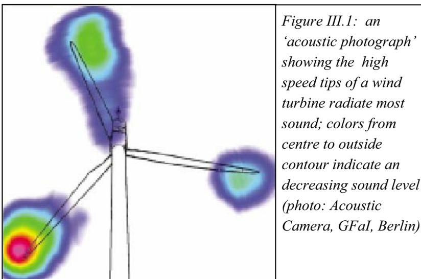
Figure III.1: an 'acoustic photograph' showing the high speed tips of a wind turbine radiate most sound; colors from centre to outside contour indicate an decreasing sound level (photo: Acoustic Camera, GFal, Berlin)
