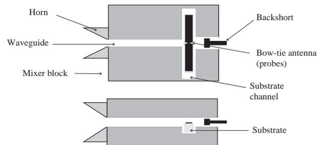
FIGURE 1.5. A schematic cross-sectional top- and side view of the mixer block with horn, backshort, substrate channel and mounted junction.
