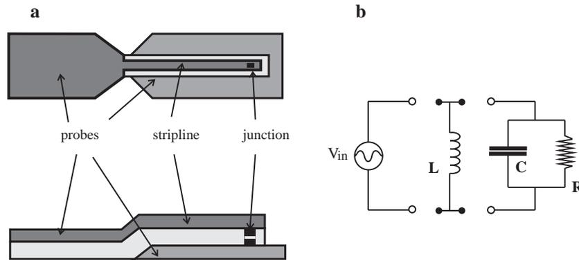
FIGURE 1.8. **a.** Top and cross-sectional view of a junction embedded in a stripline. The left probe is stretched via a narrow line over the right probe, forming a stripline. The SIS junction is situated at the end of this line. **b.** The circuit schematically shows the electrical equivalent of a stripline; the stripline acts as an inductor which cancels out the junction capacitance leaving only the real part  $R$  of the impedance.
