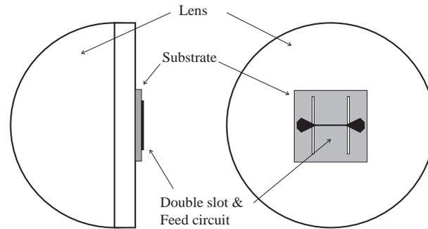
FIGURE 1.4. A simplified side- and front view respectively of the quasioptical coupling scheme; a lens with double slot antenna and coupling circuit
