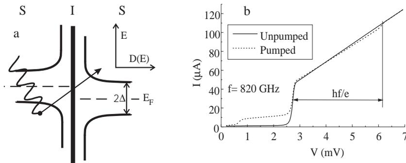
FIGURE 1.7. **a.** Energy band diagram of the SIS structure with an applied voltage. In the horizontal plane the density of states is depicted, which becomes infinite at  $|E| = \Delta$ . An incoming photon can raise the energy of a quasiparticle enabling photon assisted tunneling. **b.** The resulting current-voltage characteristics with and without 820 GHz radiation of a Nb junction.
