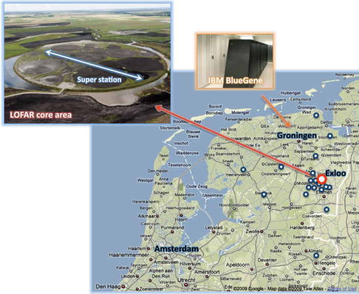
Figure 1.5: An approximate location of the LOFAR core area (red circle) and remote stations (blue circles). The data from the stations is processed in Groningen with a Blue Gene supercomputer.
