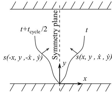
**Figure 6.5:** Definition of configurational symmetry: every ciliary configuration (i. e. the current position of all material points  $s(x, y)$  and their velocities  $(\dot{x}, \dot{y})$ ) at time  $t$  can find its mirror image after half a cycle with the symmetry plane being perpendicular to the channel.
