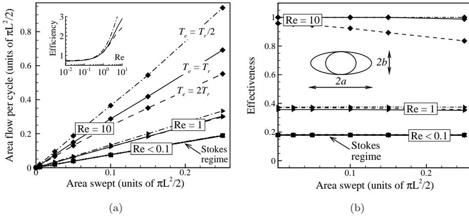
**Figure 6.2:** (a) Area flow out of the channel as a function of the area swept ( $\theta = 0^\circ$ ) for different Reynolds numbers. Also plotted are the cases in which the velocity during the effective stroke is different from that of the recovery stroke. The inset shows the efficiency of fluid flow as a function of the Reynolds number. (b) Effectiveness of fluid flow ( $(Q_p - Q_n)/(Q_p + Q_n)$ ) as a function of the area swept for different Reynolds numbers and  $T_e/T_r$  values.
