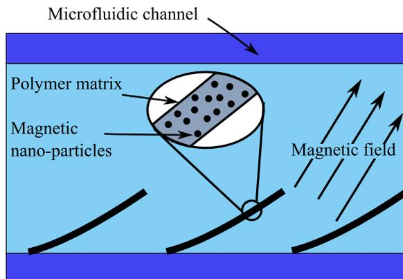
**Figure 1.3:** Schematic picture of the approach taken. The artificial cilia consist of a polymer matrix with embedded magnetic nano-particles. The cilia exhibit an asymmetric motion when a tuned external magnetic field is applied.
