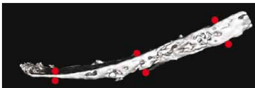
Figure 3: Lateral view of a micro-CT image of a human orbital floor sample. The red dots represent measure points for the thickness evaluation as evaluated with GE MicroView Analysis Software. The mean thickness was used for evaluation in three-point bending test.
