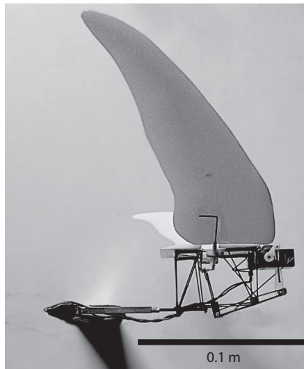
Fig. 6.1: Flapping-wing MAV mounted on the force balance. Wing-span = 0.33 m, average chord length = 40 mm, aspect ratio = 8.3 .
