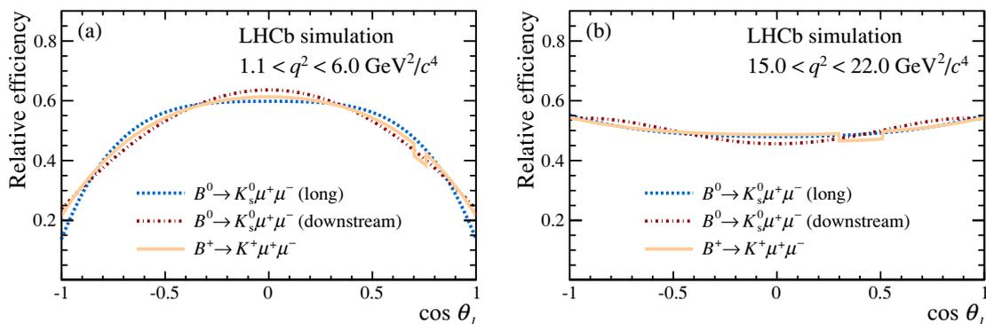
**Figure 1.** Angular acceptance as derived from simulation in the dimuon mass squared ranges (a)  $1.1 < q^2 < 6.0 \text{ GeV}^2/c^4$  and (b)  $15.0 < q^2 < 22.0 \text{ GeV}^2/c^4$ . The dip in the acceptance for  $B^+ \rightarrow K^+ \mu^+ \mu^-$  decays results from the veto used to reject  $B^+ \rightarrow \bar{D}^0 \pi^+$  decays (see text). The acceptance is normalised to unit area to allow a comparison of the shape of the distributions.
