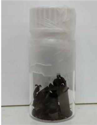
**Figure 6.1** The photograph of GO after drying
