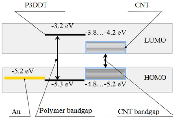
Fig. 4. Energy bands: Au-P3DDT-nanotube (with a bandgap)
