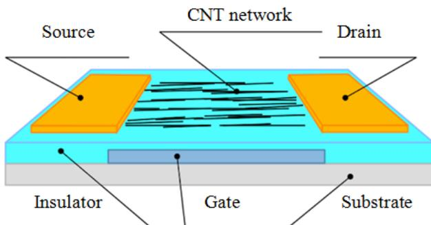
Fig. 1. The device - FET based on nanotubes network.
