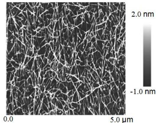
Fig. 2. Photo of FET channel (CNT network).
