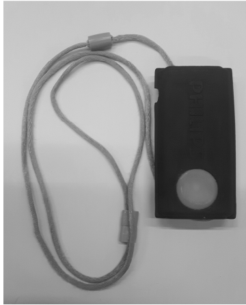
Figure 1. Senior Mobility Monitor (SMM). The device was worn in front of the chest using a provided necklace. The SMM contains a tri-axial-accelerometer and a barometer (approximate device size: 39 x 12 x 63 mm).
