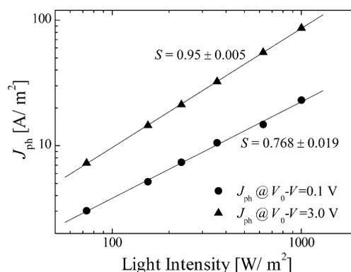
**Figure 9.** Light-intensity dependence of the photocurrent ( $J_{\text{ph}}$ ) taken from Figure 8 at an effective voltage of  $(V_0-V) = 0.1$  V and  $(V_0-V) = 3.0$  V (symbols). The slope ( $S$ ) determined from the linear fit (solid lines) to the experimental data is written on the figure.
