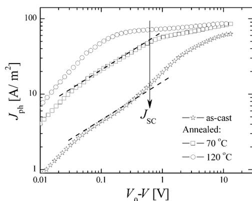
**Figure 1.** Experimental photocurrent ( $J_{ph}$ ) versus effective applied voltage ( $V_0 - V$ ) of the P3HT:PCBM devices at room temperature for as-cast devices and after thermally annealing of the photoactive layers (see legend). The thickness of the devices ( $L$ ) is 96 nm and the arrow indicates the position of the short-circuit current ( $J_{SC}$ ). The dashed lines represent the square-root dependence of the  $J_{ph}$  on voltage.
