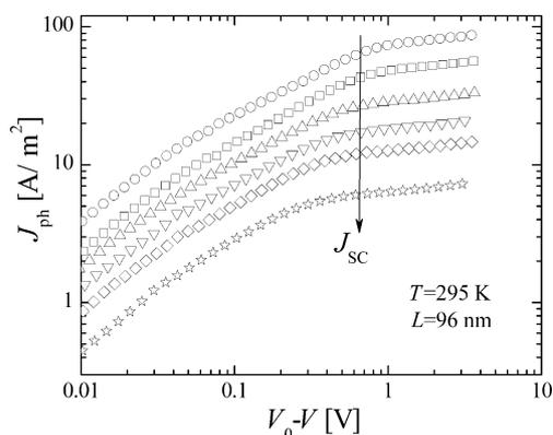
**Figure 8.** Light-intensity dependence of the photocurrent ( $J_{\text{ph}}$ ) versus effective applied voltage ( $V_0-V$ ) of the device thermally annealed at 70 °C. The intensity was varied from 1000 (upper curve) down to 76  $\text{W m}^{-2}$ , whereas the arrow indicates the position of the short-circuit current ( $J_{\text{SC}}$ ).
