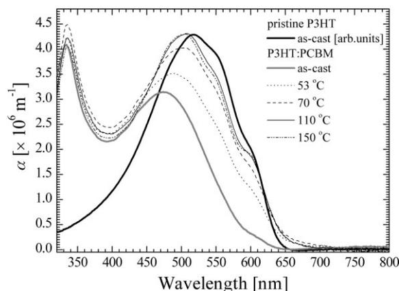
**Figure 4.** UV-vis absorption-coefficient ( $\alpha$ ) spectra of P3HT:PCBM blend films, as-cast, and for different annealing temperatures (see legend). The annealing time was 4 min. For a better comparison, the absorption of a pristine P3HT film as cast is also shown (in arbitrary units). All films were measured on a glass/ITO/PEDOT:PSS substrate and corrected for substrate absorption.
