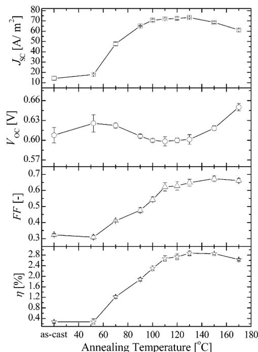
**Figure 6.** Device performance of the 50:50 wt.-% P3HT:PCBM blends, under illumination from a halogen lamp, as a function of annealing temperature. The annealing was done on a hot plate in a  $N_2$  atmosphere for 4 min. The thickness of all devices ( $L$ ) ranged from 94 to 97 nm.
