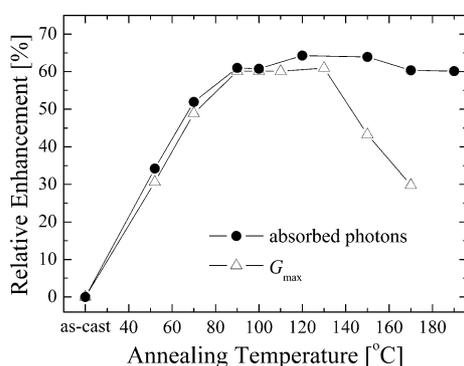
**Figure 7.** Relative enhancement [%] of the absorbed photons and maximum generation rate ( $G_{max}$ ) for an annealed compared to an as-cast device, as a function of annealing temperature. The absorption was calculated from the shaded area in Figure 5, whereas  $G_{max}$  was determined from the saturation of the photocurrent ( $J_{sat} = q G_{max} L$ ) at high effective voltages ( $V_0 - V$ ) shown in Figure 1.
