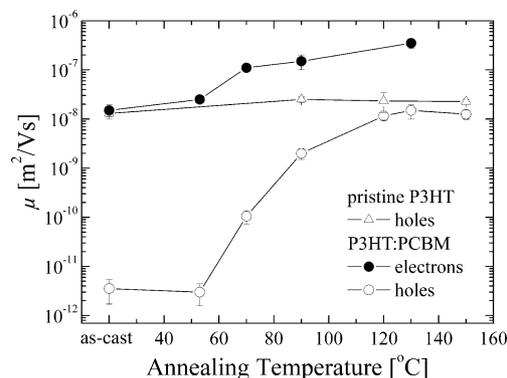
**Figure 3.** Room-temperature electron ( $\bullet$ ) and hole ( $\circ$ ) zero-field mobilities in 50:50 wt.-% blends of P3HT:PCBM as a function of postproduction annealing temperature of the completed devices. For comparison, the hole mobility measured in pristine P3HT devices ( $\Delta$ ) is also shown. The mobilities were calculated from the SCL current measured using the electron- and hole-only device configuration (Fig. 2).
