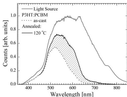
**Figure 5.** Fraction of absorbed photons ( $I_{\text{abs}}$ ) from the excitation source ( $I_0$ ) by a P3HT:PCBM solar cell with a thickness of  $L = 96$  nm. The calculation is done for the film as cast and after annealing at 120 °C (see legend) using the absorption coefficients ( $\alpha$ ) given in Figure 4.
