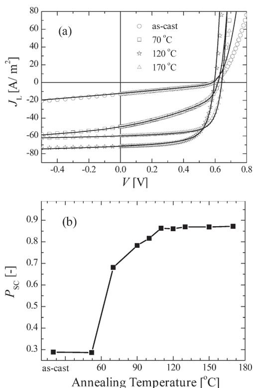
**Figure 11.** a) Room-temperature  $J_L$ - $V$  characteristics under illumination of the P3HT:PCBM devices at different annealing temperatures (symbols). The solid lines represent the numerical calculation. b) Dissociation probability ( $P_{sc}$ ) under short-circuit conditions at all annealing temperatures.
