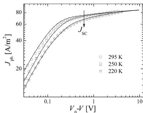
**Figure 10.** Temperature dependence of the photocurrent (symbols) versus effective applied voltage ( $V_0 - V$ ) for a 50:50 wt.-% P3HT:PCBM device with a thickness of 120 nm, annealed at 120 °C for 4 min. The solid lines represent the numerical calculation using the model form Koster et al. [16].
