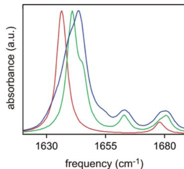
**Figure 7.** Calculated FTIR spectra of a planar AP  $\beta$ -sheet with six strands and 36 peptide groups. Normalized IR spectra are shown for calculations of (red) one ideal structure with periodic boundary conditions, (green) the same structure with open boundary conditions, and (blue) open boundary conditions averaged over random variation in position of amide I transition dipoles.
