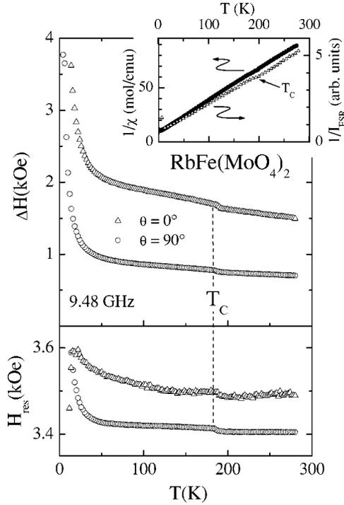
FIG. 3. Temperature dependence of the 9.48 GHz ESR linewidth (upper frame) and the resonance field (lower frame) in  $\text{RbFe}(\text{MoO}_4)_2$  for the magnetic field applied parallel ( $\theta=0^\circ$ ) and perpendicular ( $\theta=90^\circ$ ) to the crystallographic  $c$  axis. Inset: temperature dependence of the inverse ESR intensity  $1/I_{\text{ESR}}$  compared to the inverse static susceptibility  $1/\chi$ .
