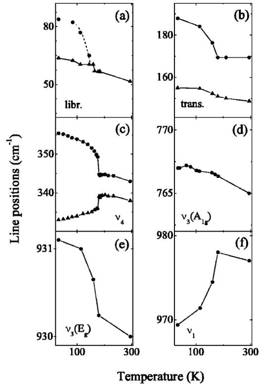
FIG. 8. Temperature dependences of Raman frequencies in  $\text{RbFe}(\text{MoO}_4)_2$ . Notations refer to the corresponding external motions and internal vibrations of the  $(\text{MoO}_4)^{2-}$  entity.
