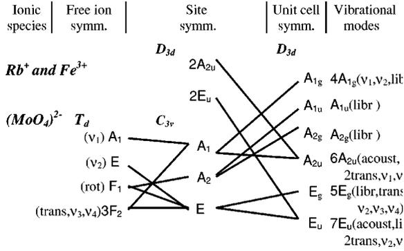
FIG. 5. Correlation scheme for vibrations of  $\text{RbFe}(\text{MoO}_4)_2$ .
