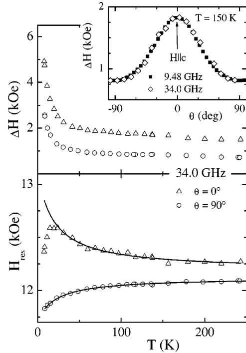
FIG. 4. Temperature dependence of the 34 GHz ESR linewidth (upper frame) and the resonance field (lower frame) in  $\text{RbFe}(\text{MoO}_4)_2$  for the magnetic field applied parallel ( $\theta=0^\circ$ ) and perpendicular ( $\theta=90^\circ$ ) to the crystallographic  $c$  axis. The solid line is obtained from the fit described in the discussion. Inset: Angular dependence of the linewidth at 150 K for both  $X$ - and  $Q$ -band frequencies.
