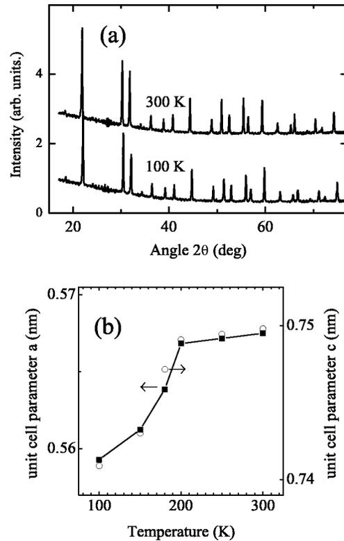
FIG. 2. Powder x-ray diffraction patterns of  $\text{RbFe}(\text{MoO}_4)_2$  at 300 and 100 K (a) and crystallographic cell parameters  $a$  (filled squares) and  $c$  (open circles) as a function of temperature (b).
