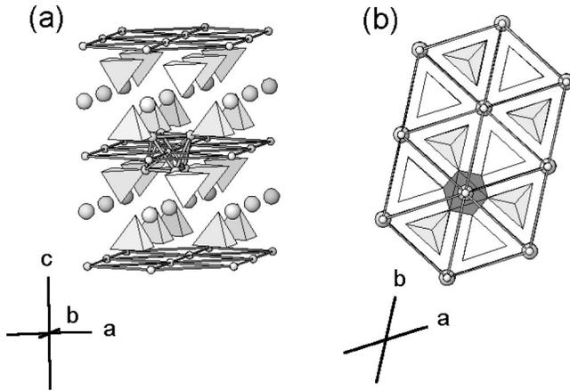
FIG. 1. Crystal structure of  $\text{RbFe}(\text{MoO}_4)_2$ . Fe and Rb atoms are represented by small and, correspondingly, big balls. Mo atoms reside within  $\text{MoO}_4$  tetrahedra (light-gray). Only one  $\text{FeO}_6$  octahedron is shown. (a) A general view. (b)  $[001]$  view.
