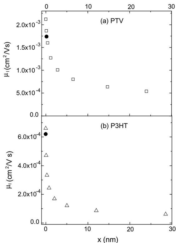
Fig. 3. The local charge carrier mobility as function of position in the accumulation layer for PTV- and P3HT-FET at  $V_G = -19 \text{ V}$  (squares for PTV and triangles for P3HT) and the extracted field-effect mobility as determined from Eq. (2) at  $V_G = -19 \text{ V}$  (dot).
