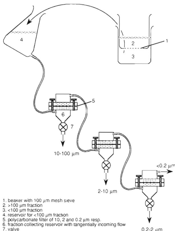
Fig. 2. Fractionation and concentration device for sea water samples, showing a cascade of tangential, reversed flow filters
