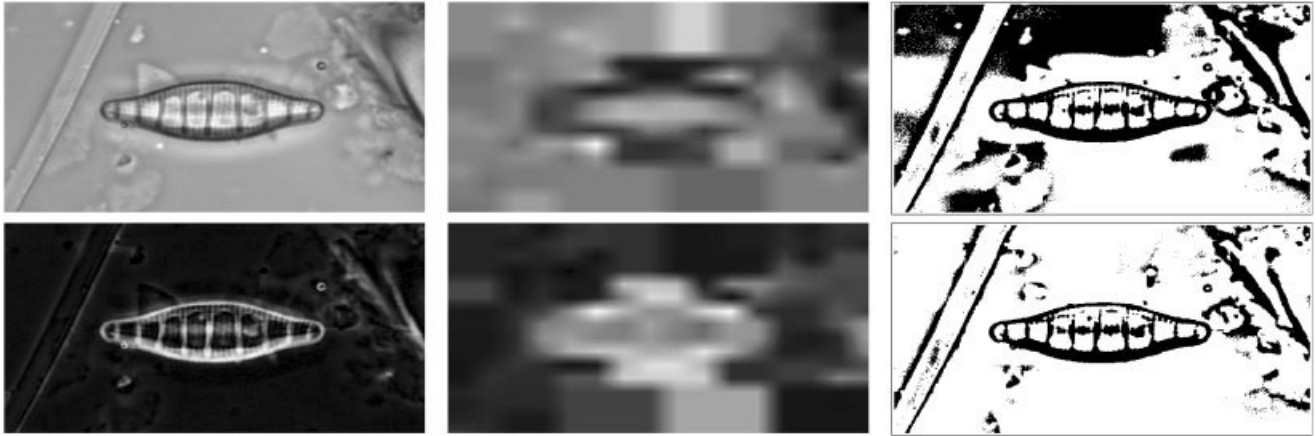
Fig. 4. RATS method. Examples. Left: Input images ( 19 \times 8 \mu\text{m} ). Middle: Threshold maps. Right: Resulting binary images. Top: No preprocessing. Bottom: After bottom-hat filtering.
