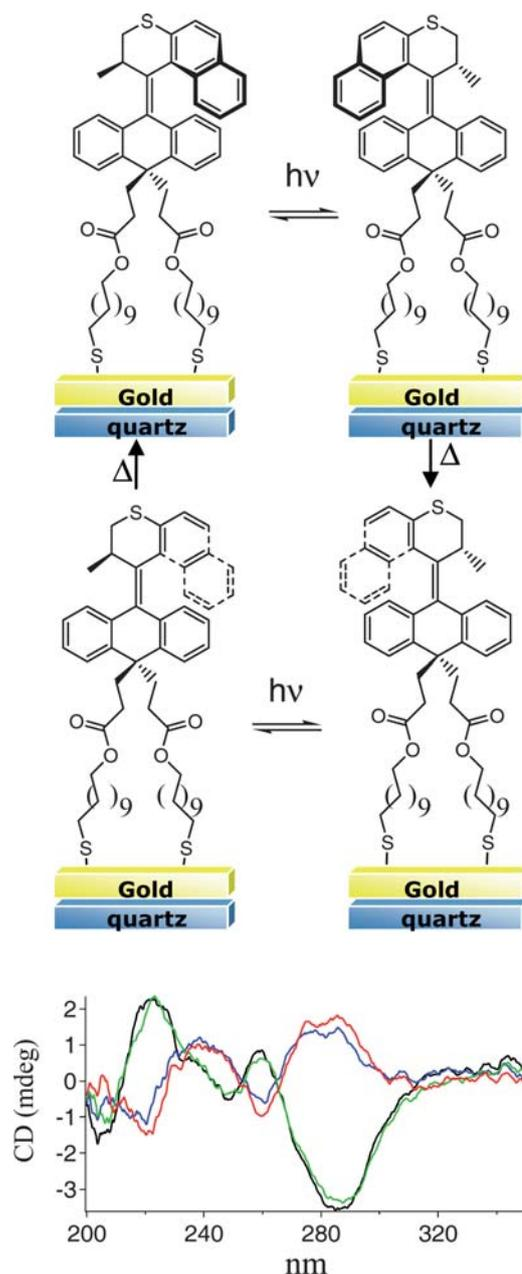
**Fig. 6** Irradiation of (2'*R*)-(M)-**3**-SAM results in a photochemical isomerization. The initial CD spectrum (black) shows an inversion of the signal as the enantiomer is generated (red). Thermal helix inversion restores the original spectrum (green). A second photochemical isomerization (blue) generates the second unstable enantiomer in the rotary cycle. Subsequent thermal helix inversion regenerates the original conformation of the motor.
