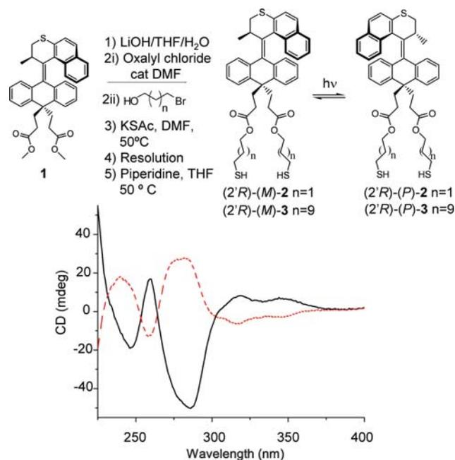
**Fig. 3** Modification of parent motor **1** with thiol-terminated linkers provides a precursor for the self-assembly of a monolayer of motors on a gold surface. The CD spectrum of (*2'R*)-(*M*)-**2** (black) in dodecane is shown. Irradiation produces the enantiomer (*2'R*)-(*P*)-**2**, which gives a CD spectrum (red) that is a pseudo-mirror image of the original due to incomplete conversion at the PSS.
