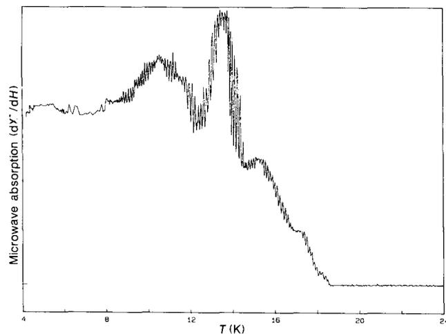
FIG. 1. Microwave loss as a function of temperature for K<sub>x</sub>C<sub>60</sub> in a static field of 20 Oe.
