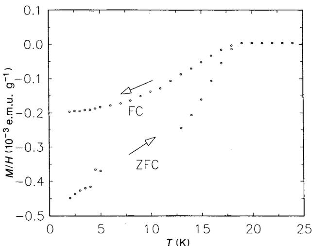
FIG. 3 Temperature dependence of the magnetization of a  $K_xC_{60}$  crystalline sample. The direction of temperature sweep in the field-cooled (FC) and the zero-field-cooled (ZFC) curves is indicated by the arrows.
