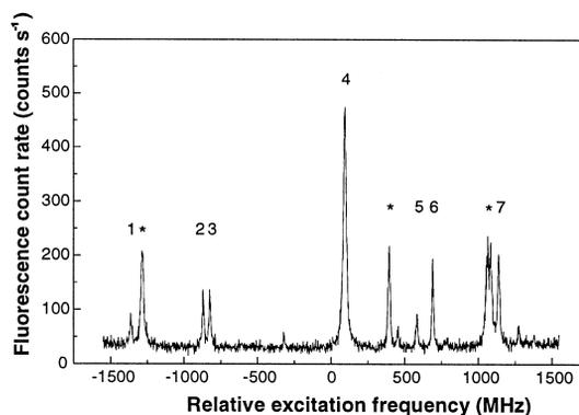
Fig. 1. Part of the fluorescence-excitation spectrum of pentacene in *p*-terphenyl. The laser frequency has been detuned by 20 GHz to the red with respect to the centre of the O<sub>2</sub> ensemble line. The features marked with an asterisk result from two or more molecules and are not considered in the evaluation.
