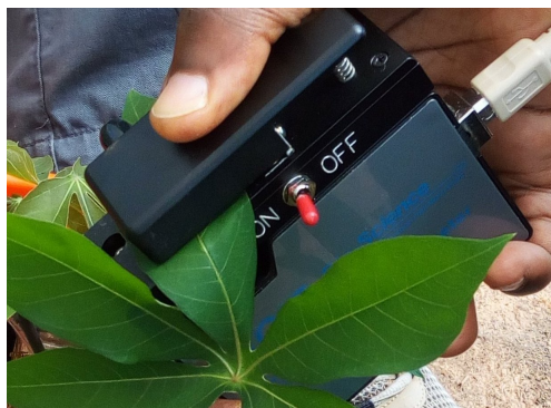
Figure 1: Data collection with a CI-710 miniature leaf spectrometer [12].
